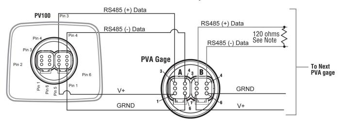
**Note:** Place Resistor between RS485+ and RS485- at end of Line on last PVA gage (included in PVJR or factory purchased panels).
